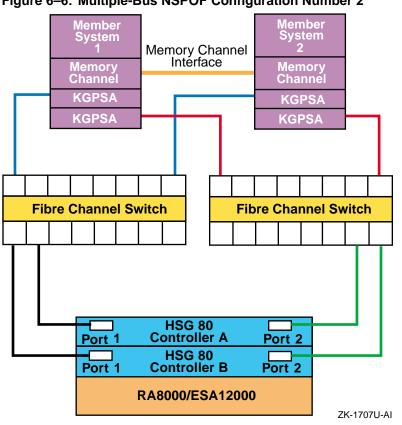
Figure 6-6: Multiple-Bus NSPOF Configuration Number 2
